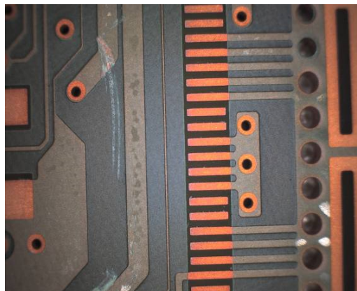
Fig. 3: mechanical solder mask defects
